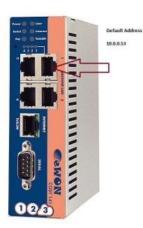
Begin configuration of your router by Connecting a CATX network cable to one of the eWONs 4 LAN side switch ports. This cable does NOT have to be a cross cable.
